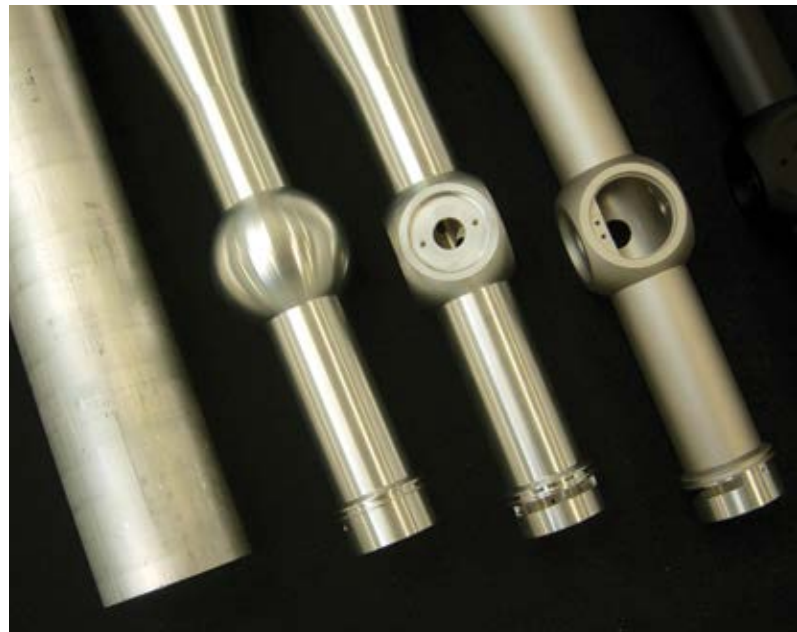
ABOVE: A technician completes erector assemblies. The variable scope's power ring engages those spiral slots. BELOW: Left to right, steps in machining a scope tube from a thick-walled blank. CNC machines hold close tolerances.
