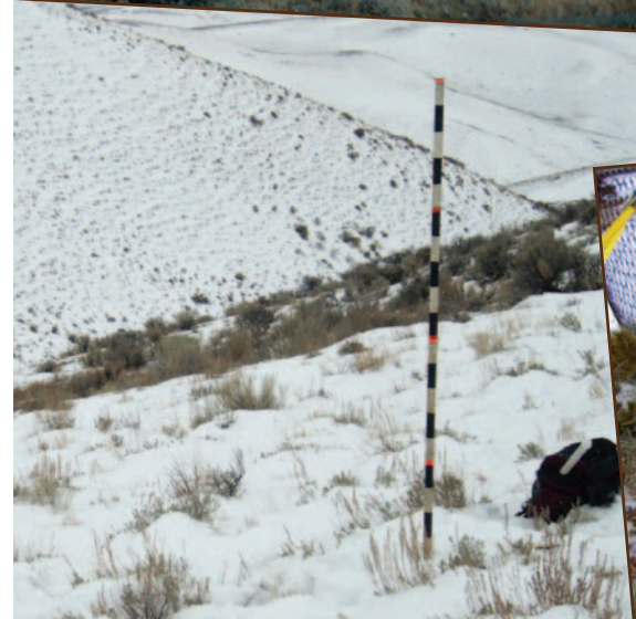
ABOVE: A cover pole used to estimate the value of hiding cover for deer.
