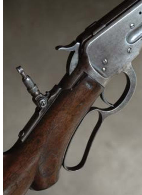
The tang sight on this early Winchester 92 makes hitting easier. A popular option back in the day!
