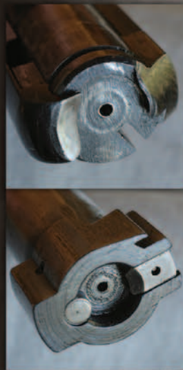
TOP: An early bolt face shows Mauser-style extractor, ejector slot, and lug tapered for coned breech. BOTTOM: This 1970s era bolt face shows face-mounted extractor, plunger ejector, and split lug for anti-bind rail.
