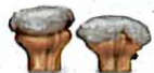
Swift A-Frame bullet reliably mushrooms to 2-X caliber, with over 95% weight retention.
