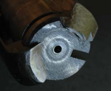
ABOVE: This early Model 70 bolt face shows its stout Mauser extractor and slot for the mechanical ejector. BELOW: “The best hunting-rifle trigger ever,” said gun guru Don Allen of the original M70’s. Wayne agrees.
