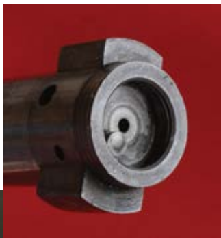
LEFT: The 721/722 rifles (1948) were economical but stout, “three rings of steel” around the cartridge head.
