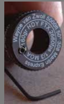
This GreyBull elevation dial permits dead-on hold at long range—with this .308 ME load only.
