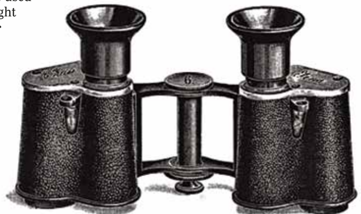
BELOW: In 1894 ZEISS developed the first binoculars with increased distance between the objective lenses for enhanced three-dimensional vision at long range.
