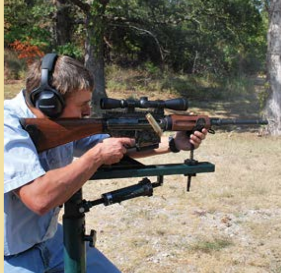
A portable bench from RCBS. Portable benches like this are extremely useful, but it's very difficult to replicate the rock-steady stability of a heavy, permanent bench weighing several hundred pounds.
