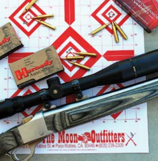
Three sub-half-inch groups fired with a Ruger No. One in .204 Ruger. Light-recoiling rifles are much easier to shoot at the bench, and three-shot groups are easier to hold than five-shot groups.
