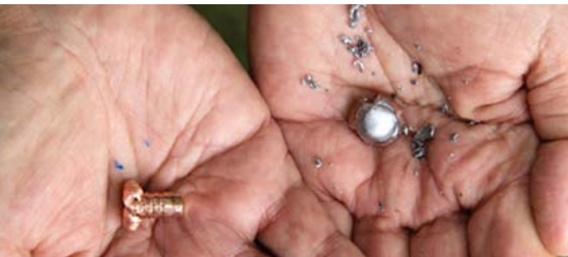
Copper solid mushroomed bullet on left; fragmented lead bullet on right.
