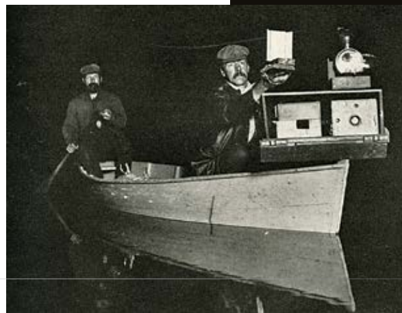
These flashlight photo hunters in 1893 were the pioneers of the sport. The hunting skiff and equipment went out for game with two cameras in the box on the revolving table in the bow. On top was the jacklight which located the game. The flashlight in Shiras’ hand was fired by pulling on a trigger. The flashlight apparatus shown was the one used in practically all the author’s night pictures of deer and moose taken from a canoe.
